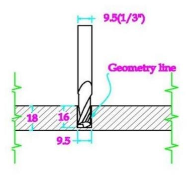
1 Use MC9.5SUC (9.5mm "up cut" cutter) Cut along outside of geometry line. Cut 16mm deep.
