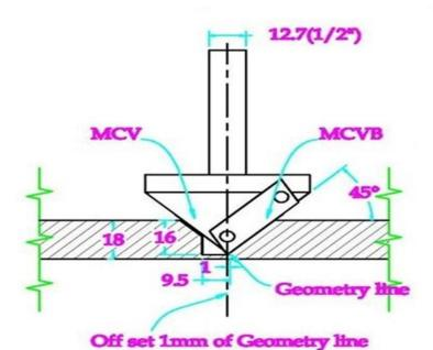
2 Use MCV (45° Vee shape cutter). Cut on centre line of offset line with 1mm offset towards geometry line. Cut 16mm deep in 2 passes recognising amount of material to be machined. Last cut is 5mm.
